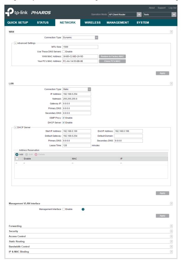
If you've made any change of the parameters, click **Apply** to make the configuration take effect. There will be a blue bar at the top of the page to remind you to save the configuration. Click **Save Changes** when you finish all settings, otherwise all the settings will be recovered to last saved settings at reboot or power off.
