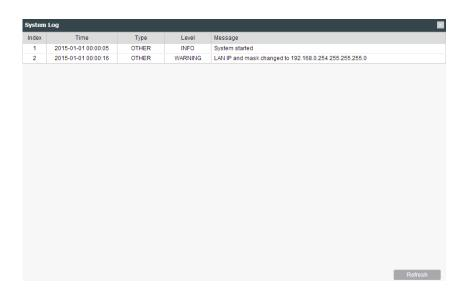
This page displays detailed system logs that can be sorted on columns by ascending or descending order. Columns can be chosen from Time, Type, Level, and Message.
