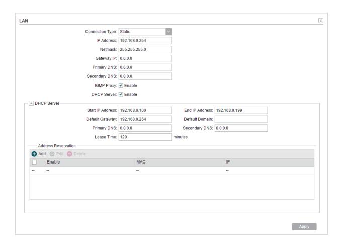
While the page of **Access Point** mode, **Client** mode, **Repeater (Range extender)** mode and **Bridge** mode is shown as below. There are two connection types including dynamic and static.
