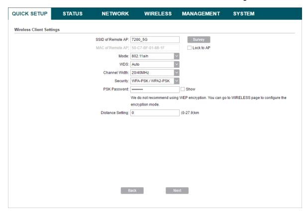
5. Create a new *SSID* and *PSK password* for the local wireless network. The wireless AP settings for the local network will be set the same as your root AP by default. Click **Next**.
