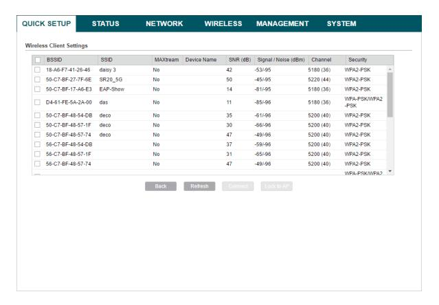
4. If the root AP needs password to be connected, you should select the same Mode, Channel Width and Security type and enter the same PSK Password as entered on the root AP. Enter the distance between this device and the root AP/router in Distance setting. Then click Next.
