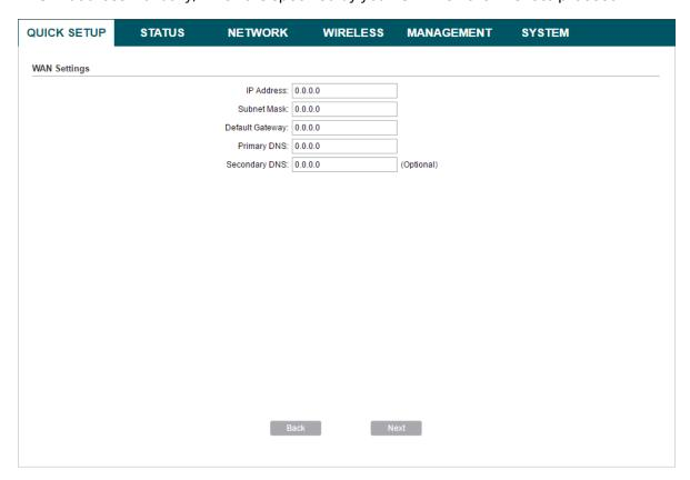
3. After configuring WAN connection type, the Wireless AP Settings page will appear as shown below. Create an easy-to-remember name for your wireless network. We recommend to select WPA-PSK/WPA2-PSK in the Security box and enter the PSK Password below to prevent unauthorized access to your AP. Enter the distance between this device and the furthest client in Distance Setting. Then click Next.
