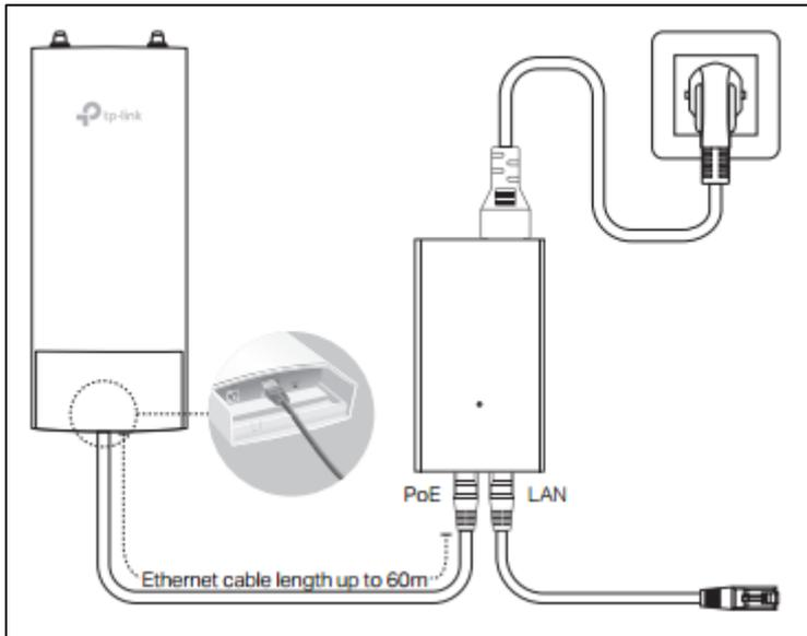
Note: Passive PoE is different from Standard PoE. You cannot supply power to EAP Outdoor products with PoE switches. For detailed information about PoE power supply, please refer to [FAQ-906](#).
