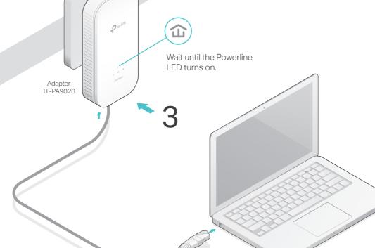
More: To add additional powerline adapters and extenders with the default settings, simply plug them into the wall sockets on the same electrical circuit.
