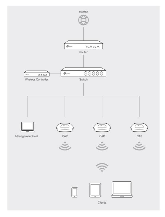
• The wireless controller can be in the same or different network segment as the CAPs.
