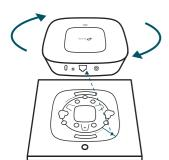
Attach the CAP to the mounting bracket by aligning the arrow mark ▼on the CAP with the arrow mark ↓ on the mounting bracket, then rotate the CAP until it locks into place, as shown on the left.
