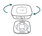
Attach the CAP to the mounting bracket by aligning the arrow mark ▼ on the CAP with the arrow mark on the mounting bracket, then rotate the EAP until it locks into place, as shown on the left.
