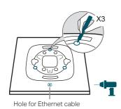
Place the mounting bracket in the center of the ceiling tile. Mark three positions for the screw holes and a position for the Ethernet cable hole.
