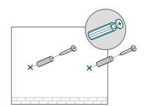
Insert the plastic wall anchors into the 6mm holes and drive the self-tapping screws into the anchors. Do not drive the screws all the way in and leave enough clearance to hang the CAP.
