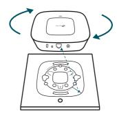
Attach the EAP to the mounting bracket by aligning the arrow mark ▼ on the EAP with the arrow mark ↓ on the mounting bracket, then rotate the EAP until it locks into place, as shown on the left.
