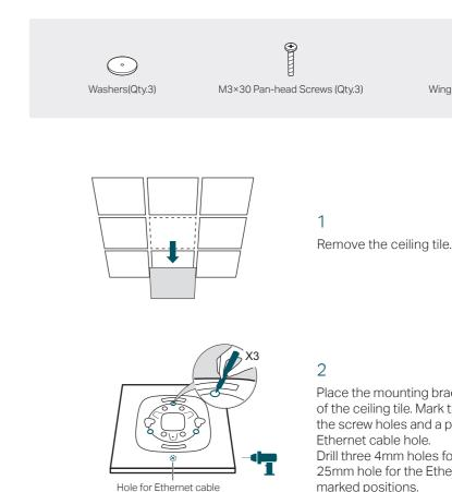
Place the mounting bracket in the center of the ceiling tile. Mark three positions for the screw holes and a position for the Ethernet cable hole.
