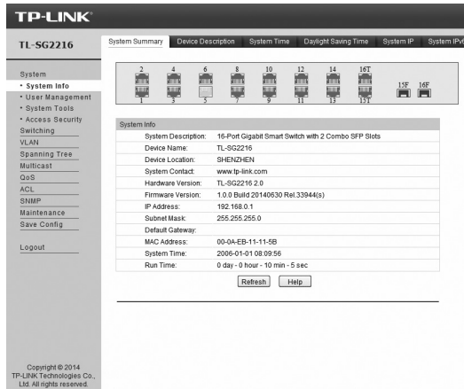
Figure 5-3 Main Page of the Switch
