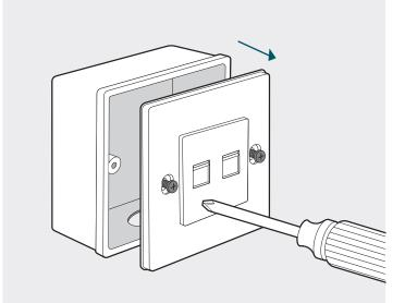
2. Detach the faceplate of the EAP with a screwdriver.
