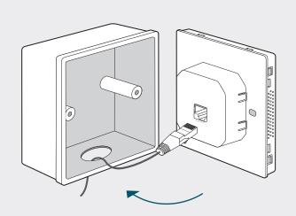
If the junction box does not have enough room to accommodate the EAP without straining the Ethernet cable, replace the junction box with an open-end or deeper one.
