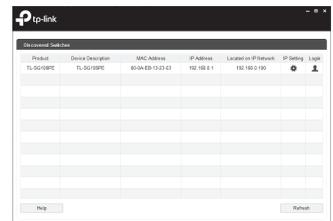
4. Make sure the switch that you want to manage is in the same subnet as your computer. You can click to configure the switch IP address.
