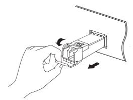
4. Reinstall the protective dust plug in the SFP's optical bores and place it on antistatic mat or a static shielding bag.
