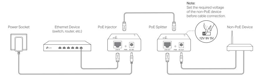
Note: TL-POE200 Power over Ethernet Kit is not compliant with IEEE 802.3af standard. The PoE Injector and PoE Splitter can only be used together. Pairing TL-POE200A or TL-POE200B with any other devices is dangerous.
