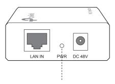
**Steady green** indicates that the power adapter is working properly.
