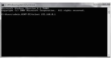
Figure 5-6 Connecting to the Switch
