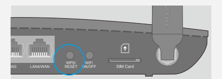
WPS/RESET Button - Press and hold until the Power LED starts flashing.
