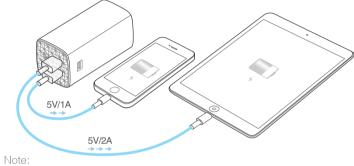
The 5V/2A USB port can automatically adjust its current to charge your 5V/1A devices.
