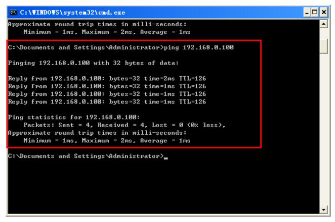
If Ping proceeds successfully and gets replies from the host in TL-ER6120, the IPsec connection must be working properly now. If there are any further problems, please feel free to contact our TP-LINK technical support.
