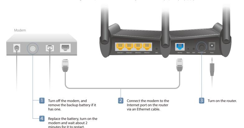
Connect your device to the router and check the LED lights.
