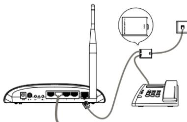
**Note** If no telephone is needed, please connect the ADSL port of the Router to the wall jack using the telephone line directly.
