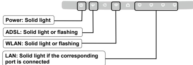
**Note** If the LEDs display abnormally, please check to see if all the cable connectors (power adapter, phone line and Ethernet cable) are well connected to your device. With the phone line well connected, if the ADSL LED turns off after flashing, please contact your ISP to ensure that your internet connection is active.
