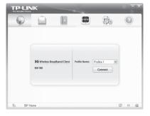
The network parameters will be configured automatically according to the SIM/USIM card inserted. With successful configuration, a profile name (your ISP name by default) will appear on the interface. Here we use Profile 1 as an example.
