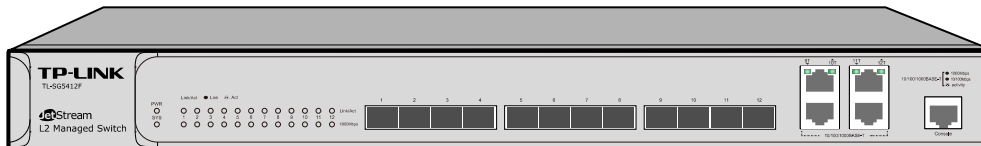
Figure 2-2 Front Panel of TL-SG5412F
