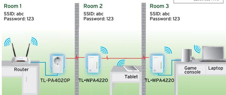
\*The Powerline Adapters need to be connected in the same electrical circuit.
