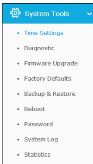
Choose menu “**System Tools**”, and you can see the submenus under the main menu: **Time Settings**, **Diagnostic**, **Firmware Upgrade**, **Factory Defaults**, **Backup & Restore**, **Reboot**, **Password**, **System Log** and **Statistics**. Click any of them, and you will be able to configure the corresponding functions. The detailed explanations for each submenu are provided below.
