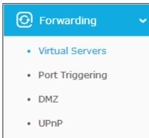
There are four submenus under the Forwarding menu: **Virtual Servers**, **Port Triggering**, **DMZ** and **UPnP**. Click any of them, and you will be able to configure the corresponding function.
