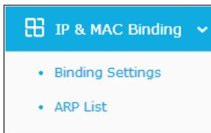
There are two submenus under the IP & MAC Binding menu, shown in the figure above: **Binding Settings** and **ARP List**. Click any of them, and you will be able to scan or configure the corresponding function. The detailed explanations for each submenu are provided below.
