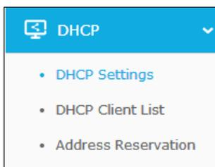
There are three submenus under the DHCP menu, shown in the figure above: **DHCP Settings**, **DHCP Clients List** and **Address Reservation**. Click any of them, and you will be able to configure the corresponding functions.
