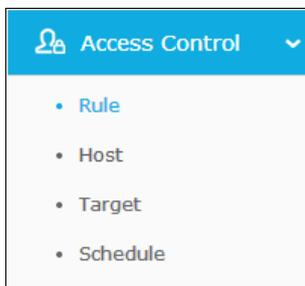
There are four submenus under the Access Control menu as shown in the figure below: **Rule**, **Host**, **Target** and **Schedule**. Click any of them, and you will be able to configure the corresponding function.
