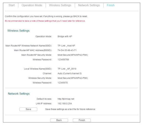
4. Relocate the access point to a good place. Connect your wireless devices to the Wi-Fi network using the access point's SSID and password.
