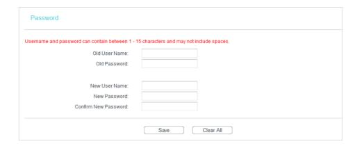
It is strongly recommended that you change the default username and password of the access point, for all users that try to access the access point's web-based utility or Quick Setup will be prompted for the access point's username and password.
