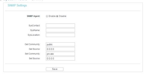
SNMP Agent - Select the radio button before Enable will enable this function if you
