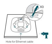
Place the mounting bracket in the center of the ceiling tile. Mark three positions for the screw holes and a position for the Ethernet cable hole.
