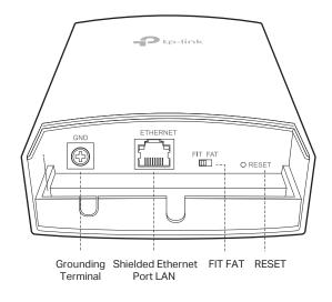
The Grounding Terminal is used for lightning and ESD protection. Use a grounding cable to connect the Grounding Terminal to earth ground.
