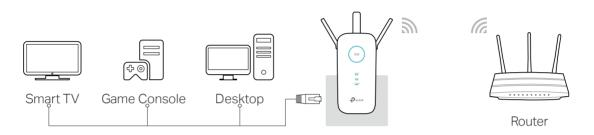
By default, the Ethernet port of the extender is connected to the 5GHz wireless netwok.
