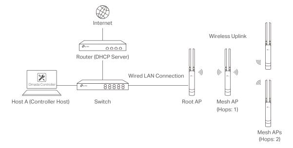
After all the EAPs are adopted, a mesh network is established. Then the EAPs connected to the network wirelessly also can broadcast SSIDs and relay network traffic to and from the network through the uplink AP.
