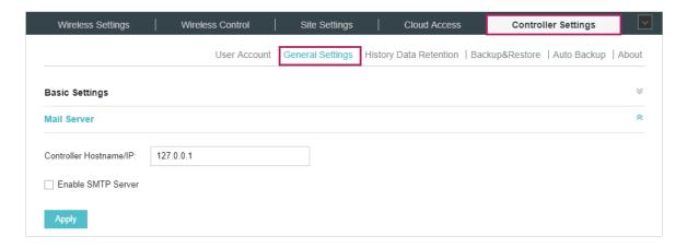
2. Enter the hostname or IP address of the Omada Controller. The default IP address of the Omada Controller is 127.0.0.1. You can keep it or customize the hostname or IP address which can be visited by the Controller host.
