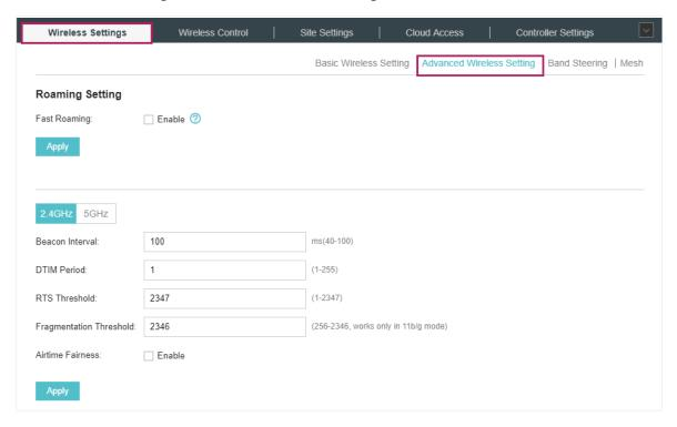
2. Enable Fast Roaming and configure the corresponding parameters.
