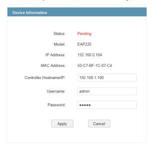
6. Click **Apply** to inform the EAP of the Controller Host's hostname or IP address. And then the connection can be established between the EAP and the Controller Host.
