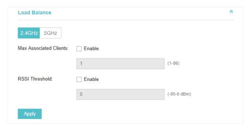
Select the frequency band (2.4GHz/5GHz) and configure the parameters.
