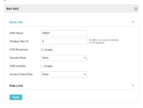
To make it easier for customers to connect, change the Security Mode from WPA-PSK to None. Customers can connect to the EAPs without password and be redirected to the Portal Authentication where the correct password will be required.
