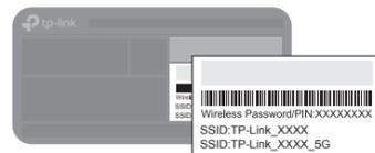
The default wireless network names (SSIDs) and password are printed on the label at the bottom of the router.
