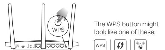
2. Within 2 minutes, press the WPS button on the extender for 1 second. The Signal LED should change from blinking to solid on, indicating successful connection.
