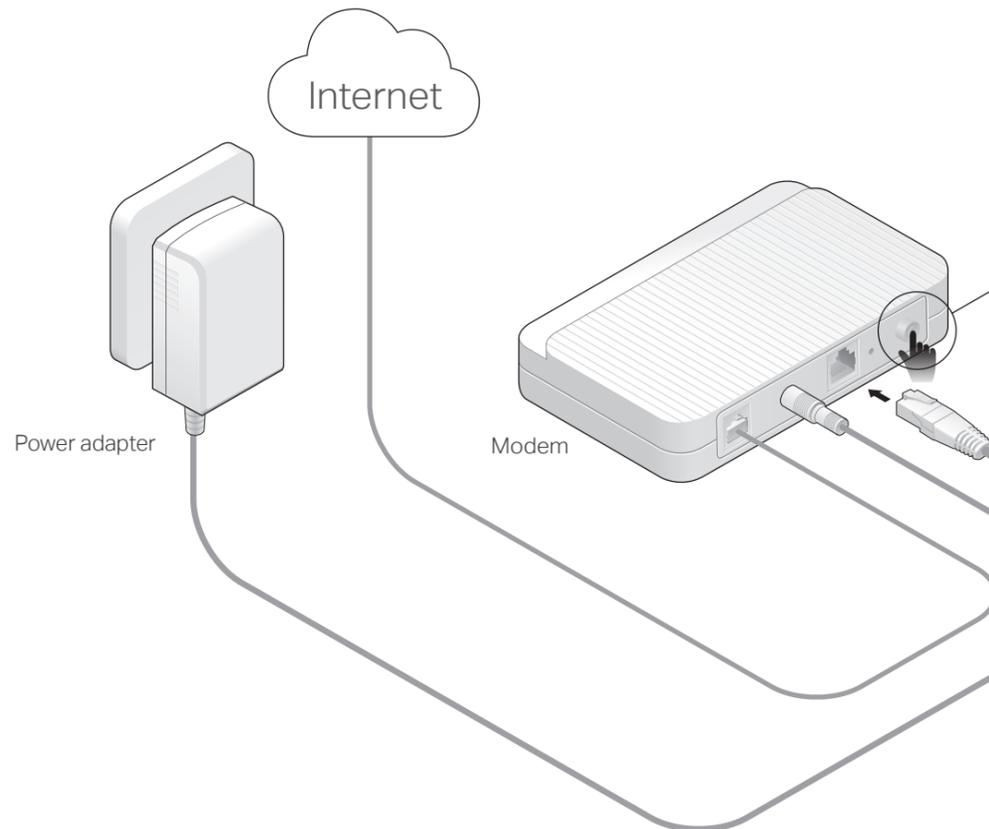
**6** Verify that the following LEDs are on and solid to confirm the hardware is connected correctly.
