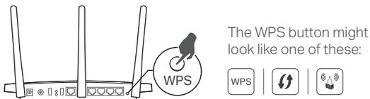
2. Within 2 minutes, press the button on the extender for 1 second.
