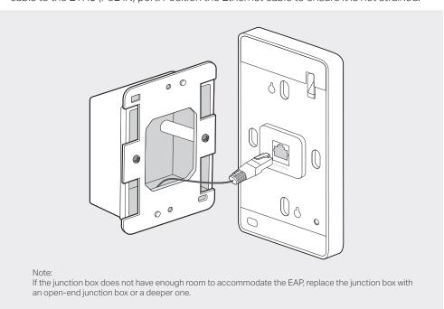
4. Attach the EAP to the mounting bracket by aligning the two mounting studs on the mounting bracket with the large openning of the slots on the EAP. Press and slide the EAP
