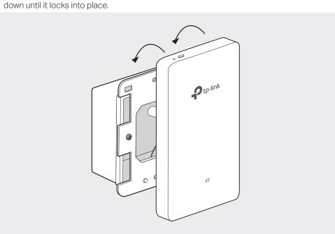
To remove the EAP from the mounting bracket, insert a paper clip into the hole next to the LED button to release the Locking Tab. Slide the EAP upwards and pull it out to detach it from the mounting bracket, as shown below.
