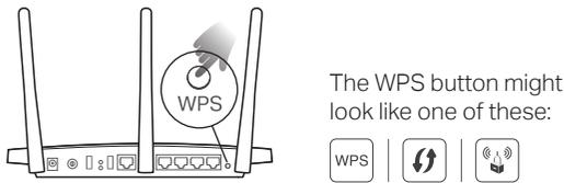
2. Within 2 minutes, press the WPS button on the extender for 1 second. The Signal LED should change from blinking to solid on, indicating successful connection.
