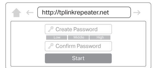
3. Follow web instructions to complete the setup. The Signal LED should turn solid on, indicating successful connection to your router.
