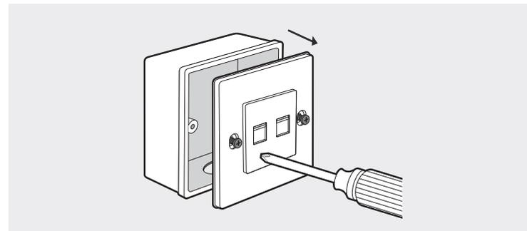
2. Detach the faceplate of the EAP with a screwdriver.
