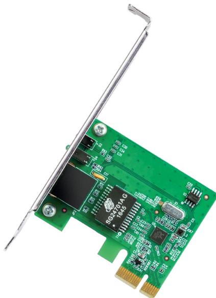
There are three LEDs, including a 10Mbps Link/Act LED, a 100Mbps Link/Act LED, and a 1000Mbps Link/Act LED. You can check the adapter's status by following the LED explanation table.
