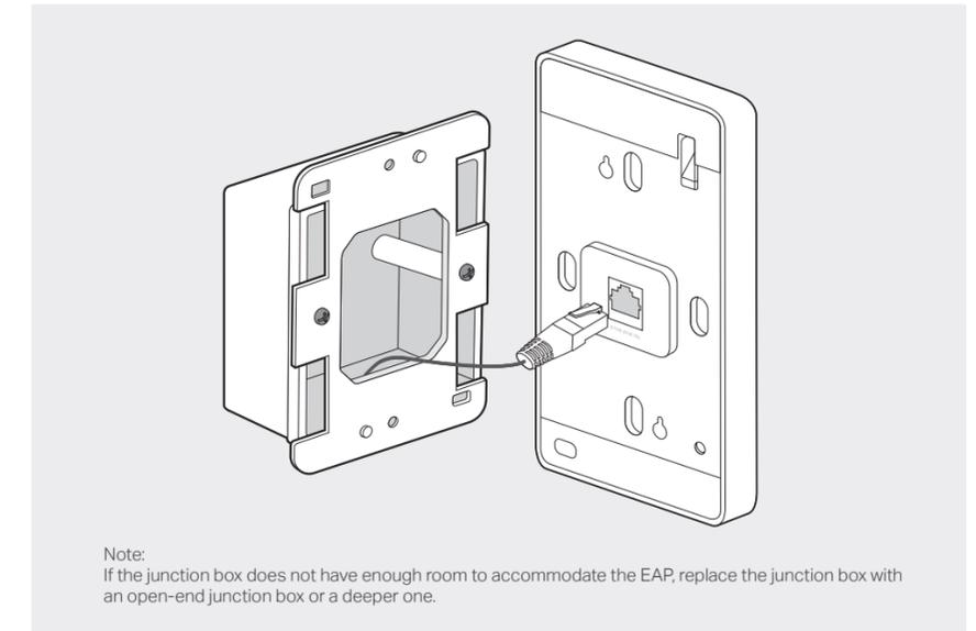
4. Attach the EAP to the mounting bracket by aligning the two mounting studs on the mounting bracket with the large opening of the slots on the EAP. Press and slide the EAP down until it locks into place.
