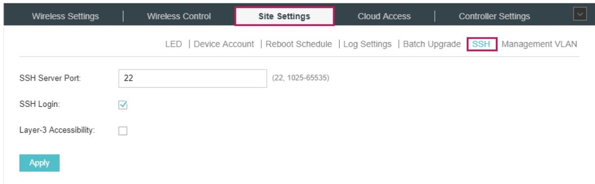
The screenshot shows the Omada Controller interface. The top navigation bar includes 'Wireless Settings', 'Wireless Control', 'Site Settings' (highlighted with a red box), 'Cloud Access', and 'Controller Settings'. Below the navigation bar, there are links for 'LED', 'Device Account', 'Reboot Schedule', 'Log Settings', 'Batch Upgrade', 'SSH' (highlighted with a red box), and 'Management VLAN'. The main content area is titled 'SSH' and contains the following configuration options:
