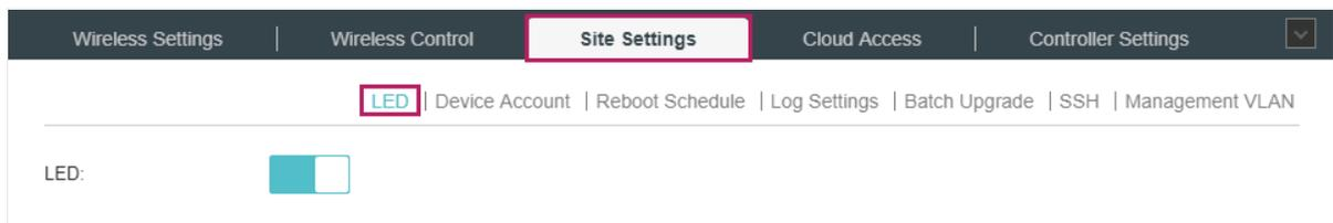
By default, the LED status is , which means that the LED lights of all the EAPs on the site are on. You can click this button to change the LED light status. The icon will be changed to , which means that all the LED lights are off.
