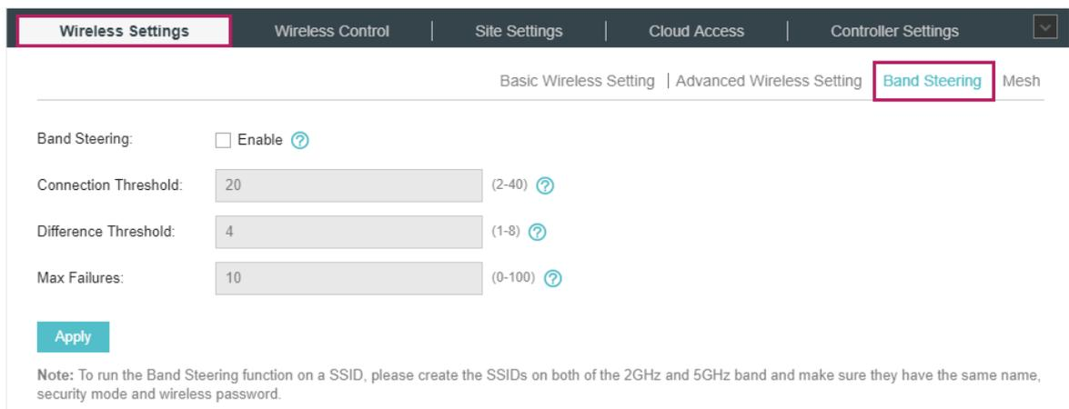
The screenshot shows the Omada Controller's configuration interface. At the top, there are navigation tabs: 'Wireless Settings' (highlighted with a red box), 'Wireless Control', 'Site Settings', 'Cloud Access', and 'Controller Settings'. Below these, there are sub-tabs: 'Basic Wireless Setting', 'Advanced Wireless Setting', 'Band Steering' (highlighted with a red box), and 'Mesh'. The 'Band Steering' section contains the following settings:
