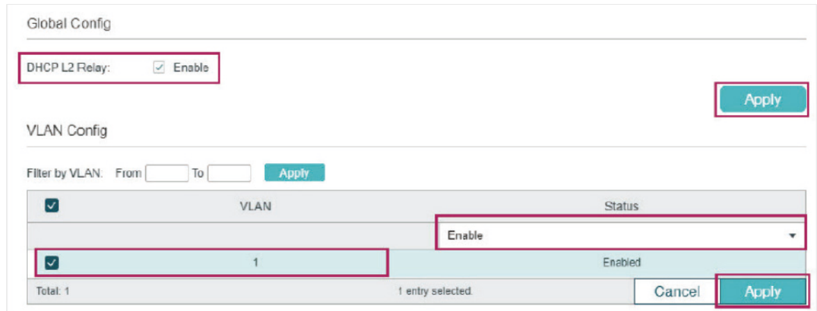
Figure 4-16 Enabling DHCP L2 Relay
