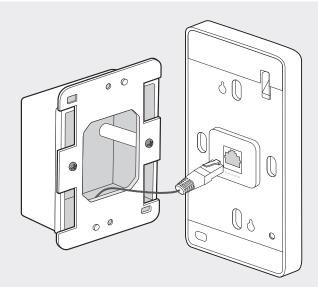
If the junction box does not have enough room to accommodate the EAP, replace the junction box with an open-end junction box or a deeper one
