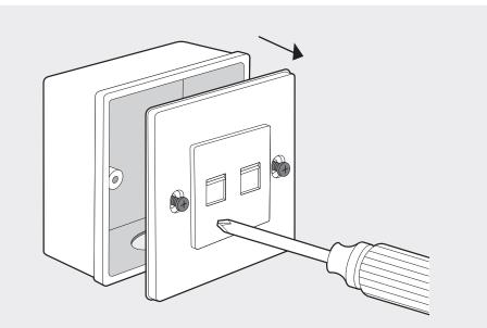
2. Insert the enclosed screws and tighten them with a Philips screwdriver to secure the mounting bracket.
