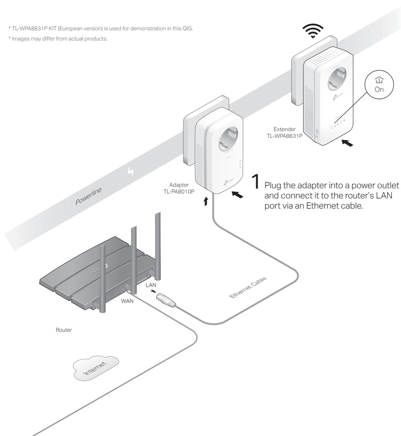
**1** Plug the adapter into a power outlet and connect it to the router's LAN port via an Ethernet cable.
