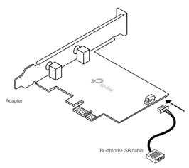
3. Locate an available PCIE X1 slot and carefully insert the adapter.
