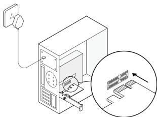
4. Locate an available F\_USB connector and carefully plug the Bluetooth USB cable into it.
