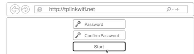
3. Run the **Quick Setup**, select **Wireless Router** and follow the step-by-step instructions to set up the internet connection.
