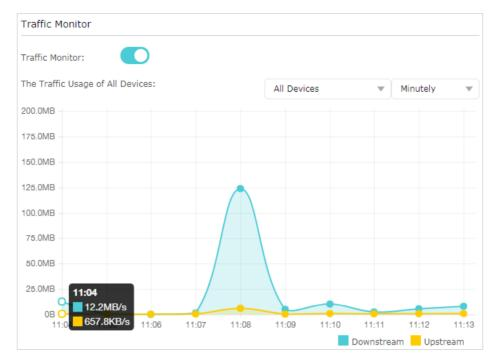
4. Check the total traffic statistics of each device on Traffic Monitor List.
