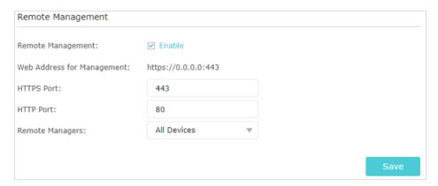
Forbid all devices to manage the router remotely:
