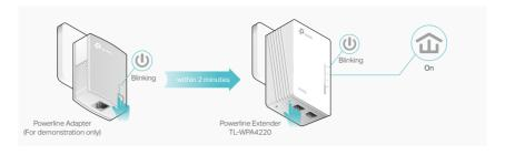
**5.** Relocate the extender to the Wi-Fi "dead" zone. Use the SSID (network name) and password on the label at the top of the extender.
