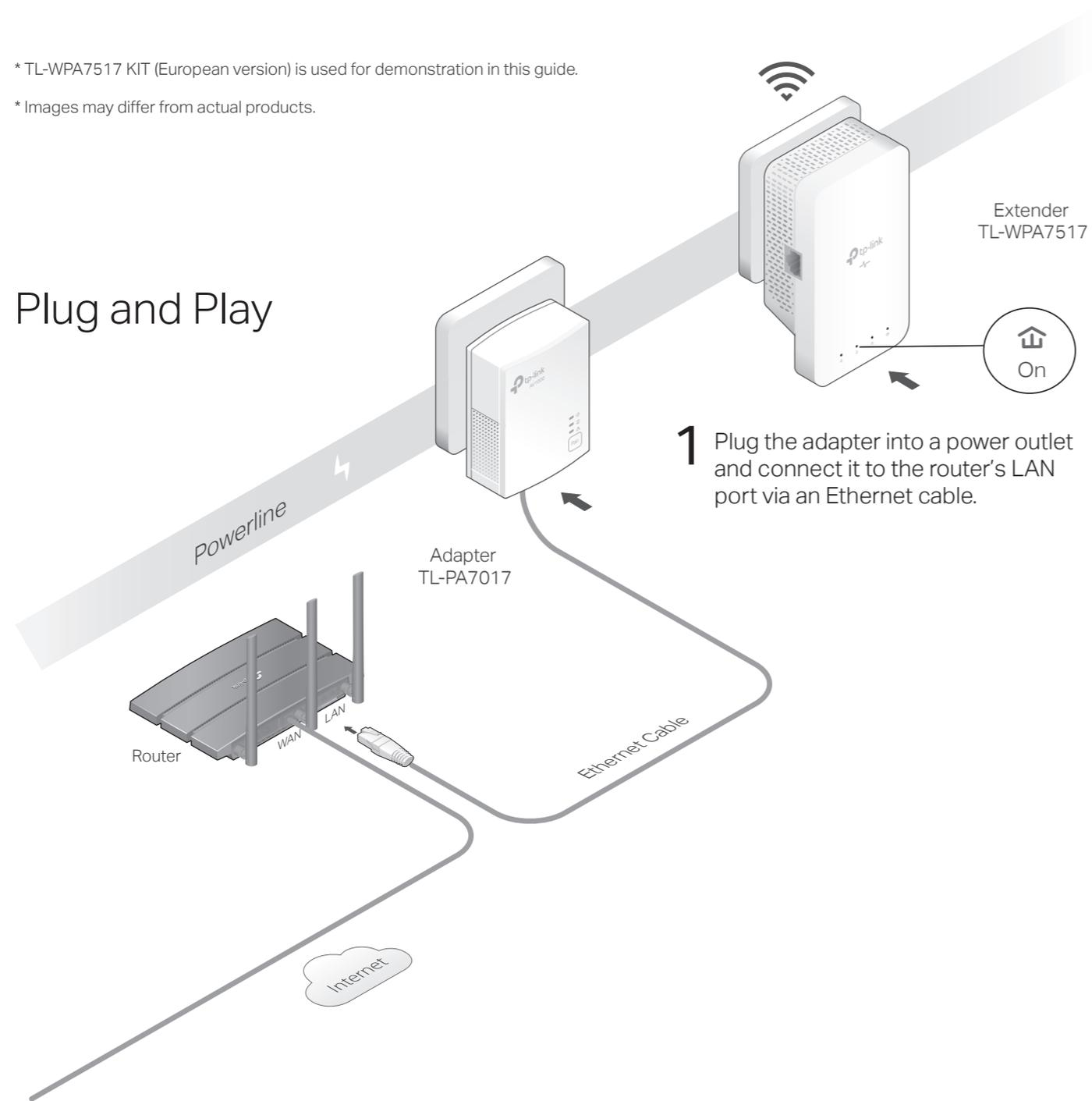
2 Plug the extender into a power outlet on the same electrical circuit. Wait until the extender's Powerline LED turns on.
