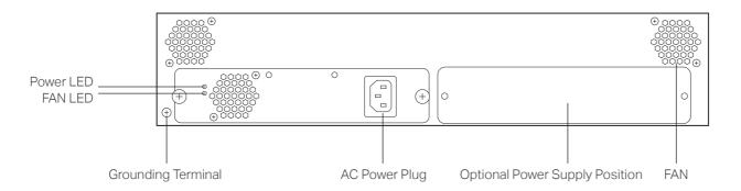
Note: An optional AC or DC power supply is available for installation in the optional power supply position.
