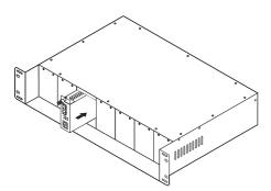
Step 2: (Optional) Install the Redundant Power Supply Module
