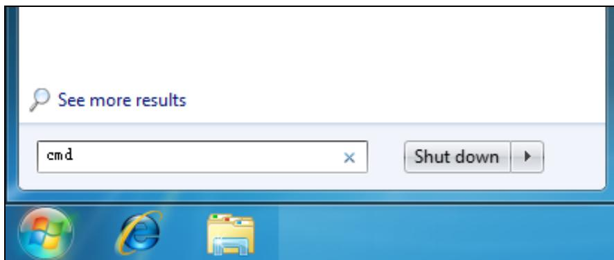
2. Type in telnet 192.168.0.1 in the cmd window and press **Enter**.
