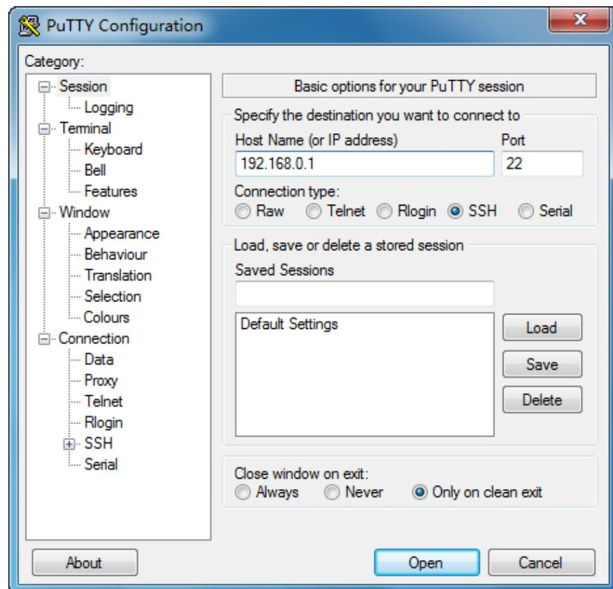
2. Click the **Open** button in the above figure to log on to the switch. Enter the login user name and password to log on the switch, and then enter enable to enter Privileged EXEC Mode, so you can continue to configure the switch.
