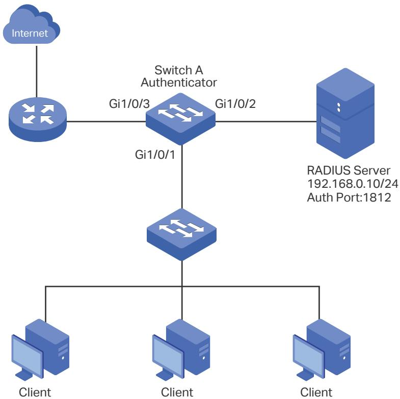
Demonstrated with T1700G-28TQ acting as the authenticator, the following sections provide configuration procedure in two ways: using the GUI and using the CLI.
