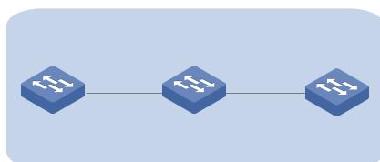
The chain topology is mainly used in a network where switches in the stack are distributively located.
