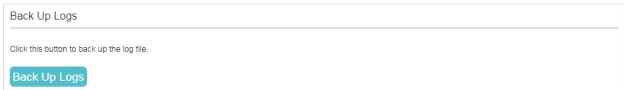
Click **Back Up Logs** to save the system logs as a file on your computer. If the switch system breaks down, you can check the file for troubleshooting.
