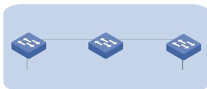
The ring topology is more reliable than the chain topology. In a chain connected stack, link failure can cause stack split. While in a ring connected stack, the system is able to operate normally with a new chain topology when a link failure occurs.
