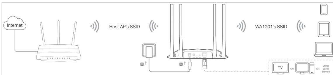
1. Connect the access point according to Step A and B in the diagram.
