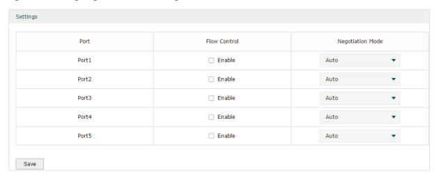
Configure the flow control and negotiation mode for a port.
