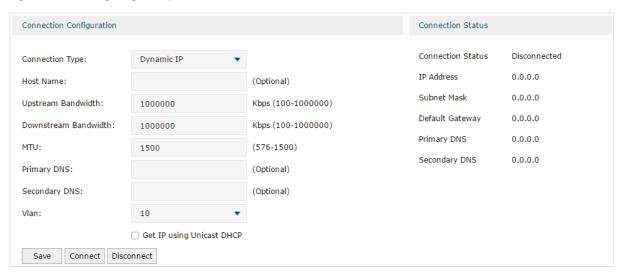
In the **Connection Configuration** section, select the connection type as Dynamic IP. Enter the corresponding parameters and click **Save**.
