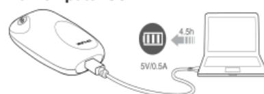
\*If the battery icon on the M5250's LED screen light on and doesn't flash any more, it means your M5250 is fully recharged.
